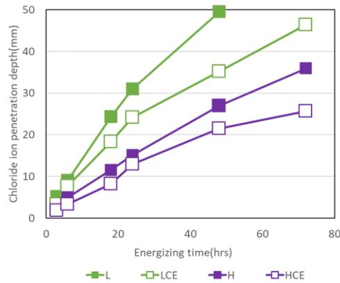
Figure 4. Chloride-ion penetration depth (using LPC and HEC mix proportion)
