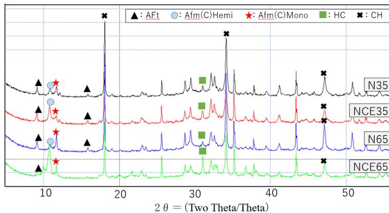
Figure 7. Diffraction results by XRD
