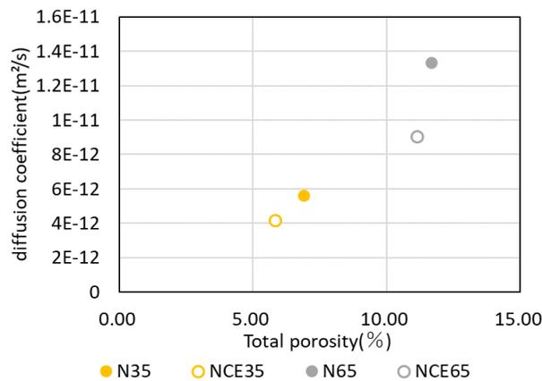
Figure 10 Relationship between porosity and diffusion coefficient
