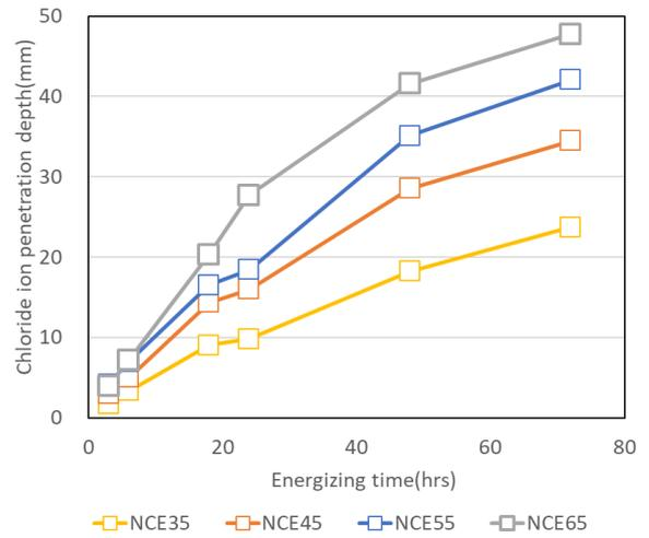
Figure 3. Chloride-ion penetration depth (NCE mix proportion)
