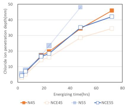
Figure 5. Chloride-ion penetration depth (W/B=45% and 55%)
