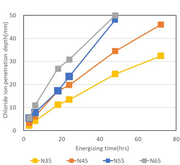
Figure 2. Chloride-ion penetration depth (N mix proportion)
