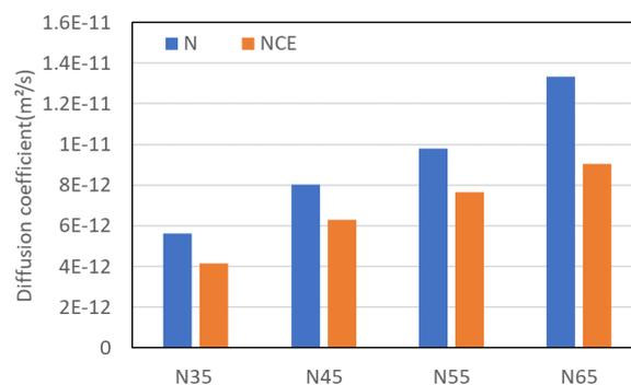
Figure 6. Diffusion coefficients for different concrete mix proportion
